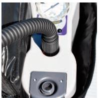
Connect the other end of the hose to the red inflation port at the top of the pump, located near the ON and OFF buttons.
