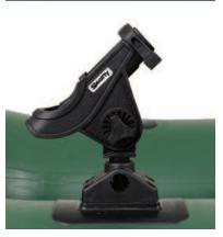
Next, install the rod holder by pushing the post straight down into the mount. Rod holder is designed to enter the mounting bracket only when pointing inboard and is locked in every other direction.
