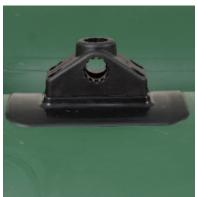
Begin by installing the side/deck mount into the glue on pads that are pre-installed on your Frameless Pontoon Boat. Be sure the "logo" on the mount reads upright when looking from inboard before securing the mount with the provided hardware.
