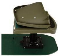
Slide the pedestal into the seat mount. Check to make sure that the spring loaded lever mechanism is locked once the seat and pedestal are installed.
